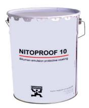
Nitoproof 10 is a brown/black liquid blend of selected bitumen emulsified with water to give an easily applied protective coating. Acts as a damp-proof membrane and vapour seal for concrete and masonry. It can also be used as a protective coating for concrete below ground.
