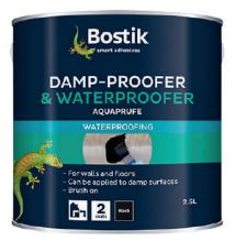
Bostik Aquaprufe Damp-Proofer & Waterproofer is a flexible, cold applied, odourless, rubber enriched bitumen emulsion for use both internally and externally. Bostik Aquaprufe Damp-Proofer & Waterproofer must be overlaid with a minimum 50mm flooring screed.
