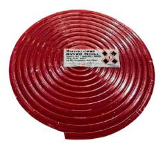
High performance swellable waterstop for in-situ concrete. Integral sealing for construction joints in concrete cast insitu. Convenient and problem solving in situations where a conventional waterstop would require complex shuttering.
