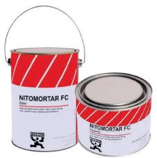
Nitomortar FC is a two component thixotropic, solvent free, compound based on epoxy resins, graded fillers and performance additives. It is applied directly to concrete substrates, without primer, and cures to a uniform smooth surface ready for over coating.
