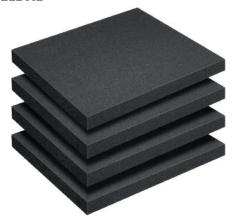
Hydrocell XL is a cross linked, non-absorbent, semi-rigid, cellular polyethylene joint filler used for forming expansion joints in concrete, brickwork and blockwork. The product provides excellent support to sealants subject to hydrostatic pressure and is particularly recommended for water retaining or water excluding structures
